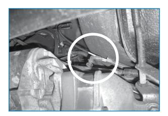
Locate the main vacuum source. This connection varies between model years. Follow the WHITE line beside the starter up to the firewall cowl to locate the main vacuum source.
