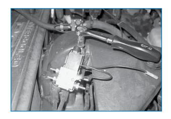
Locate transfer case vacuum lines adjacent to transmission <u>above starter on driver's side</u> of vehicle (green line = vacuum vent / white line = vacuum source)
