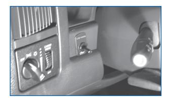
Locate a 12 volt ignition power source with a 14 to 16 gage wire diameter and connect the "T" tap terminal. Insert the male terminal of the RED wire into the "T" tap. Connect the black to a good chassis ground.
