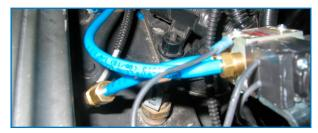
7 Using the short hose with breather vent installed, connect to port #3 of the solenoid valve. Route this breather to a location free from water and dirt.
