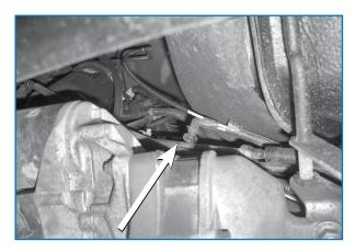
Connect the long, blue nylon, line to port #4 of the solenoid and route the other end to the elbow on the existing green line. Using the other 1/4 x 1/8 (male/female) fitting assembled in step 5, insert the larger 1/4" barbed side into the rubber 90° hose end. Connect the smaller side to the blue nylon hose from port 4 of the solenoid. Secure all hoses with tie straps provided.
