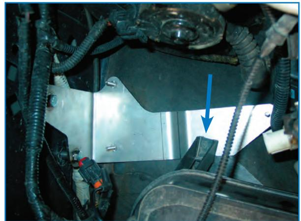
**Note: The notch in the compressor bracket must be UNDER the vacuum reservoir foot.**
