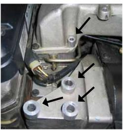
Install the compressor assembly over the 4 spacers. Obtain the best clearance of the compressor to coolant hose and compressor to intake horn as possible. Torque the 3 large capscrews (shown with arrow, under the compressor) to approximately 32 ft-lbs, (43 N•m). Torque the allen head carp screw to 18 ft-lbs 24 N•m.
