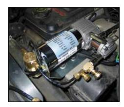
Consult with the customer for a preferred location for the quick connect airline coupler. Route the supplied airline to this location and connect to the coupler. Connect the other end to the remaining fitting at the compressor head.
