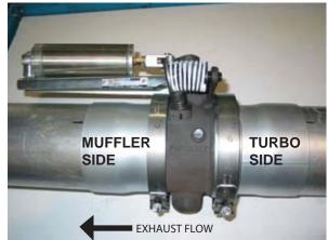
If removed, re-install the front section of pipe on the engine. Torque the turbo "V" clamp to the manufacturer's specifications. Center the Pacbrake on the pressure side adapter and install the heavy duty "V" clamp. Torque to 15 ft-lbs. Install the rear section of pipe to the Pacbrake and install the remaining "V" clamp loosely. Check the alignment of the exhaust system and adjust if necessary. Then torque both "V" clamps to 15 ft-lbs.
