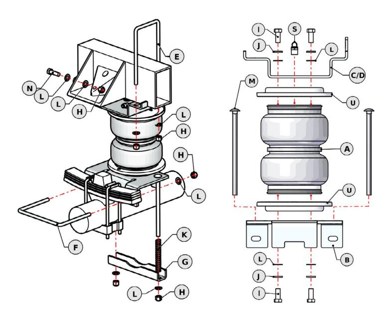
**NOTE:** Both diagrams are of the left (drivers) side of the vehicle. Reverse any orientations when assembling and installing the right (passengers) side of the vehicle.
