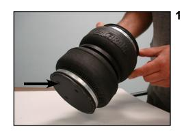
2 Place the roll plate over the end of the air spring, aligning the two mounting holes (rounded end towards the air spring). Then, place the lower mounting bracket with the flange towards you over the roll plate and air spring aligning the two mounting holes.
