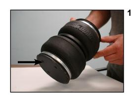
Place the roll plate over the end of the air spring, aligning the two mounting holes (rounded end towards the air spring). Then, place the lower mounting bracket with the flange towards you over the roll plate and air spring aligning the two mounting holes.
