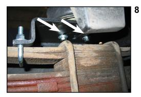
Tighten the front and rear "U" bolts around the leaf spring pack. Vehicles with overload springs use the shorter "U" bolts around the overload leaf. Vehicles without overload springs use the longer "U" bolts around the entire spring pack. Use the nylock nuts and small O.D. flat washers, torque to 16 ft-lbs. Cut off the threaded portion of the "U" bolt above the nyloc nut.
