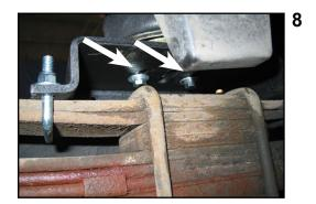
Tighten the front and rear "U" bolts around the leaf spring pack. Vehicles with overload springs use the shorter "U" bolts around the overload leaf. Vehicles without overload springs use the longer "U" bolts around the entire spring pack. Use the nylock nuts and small O.D. flat washers, torque to 16 ft-lbs. Cut off the threaded portion of the "U" bolt above the nyloc nut.
