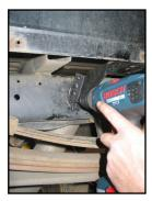
Reinstall the lower air spring assembly. Using the %" x 1/6" capscrews, flat and lock washers loosely fasten the top of the air spring to the upper bracket. Install the correct "U" bolts around the leaf spring and through the two holes in the lower bracket. Adjust the air spring on their brackets to achieve correct alignment. Once the correct alignment is achieved, tighten the upper and lower brackets to the air spring. Torque to 20 ft-lbs.
