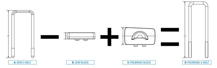
If the sum of measurement A and C, minus measurement B, is equal or less than to the length of the new U-bolts (A-B+C=D), then you can proceed with the installation.
