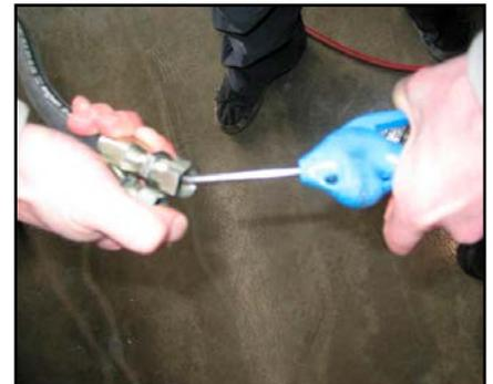
**10** Install the oil lines from the replacement filter head assembly to the new remote filter head as determined in Step 7. If necessary, secure the lines with the tie-straps provided, protecting the oil lines from heat sources and moving parts.
