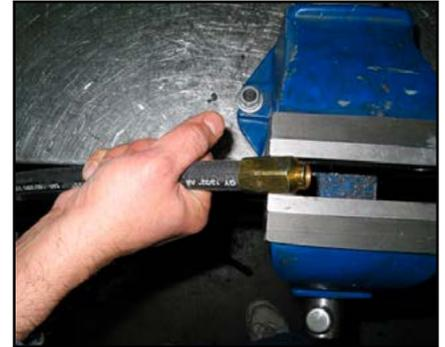
**9** **VERY IMPORTANT:** Blow out the lines from each end with shop air to remove all debris. Check the volume of air exiting each to ensure no restrictions exist.
