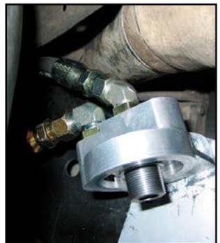
**8** With the oil supply and return lines cut to length, install the compression fittings. Install the outer nut of the compression fitting into a vise, insert the end of the line turning it counter clockwise until it bottoms, then turn it back (clockwise) ½ turn. Apply clean engine oil to the taper and threads of the inner compression fitting then screw the nipple assembly into the outer nut using a wrench until the nipple shoulder contacts the outer nut. Repeat on both ends of each oil line.
