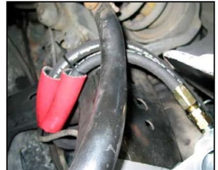
**11** Install a new oil filter. It is a good idea to fill the new oil filter with clean engine oil prior to installation. The Pacbrake remote filter head is designed for use with the factory part number oil filter. Double check all the fittings to ensure they are tightened adequately before moving to Step 12.
