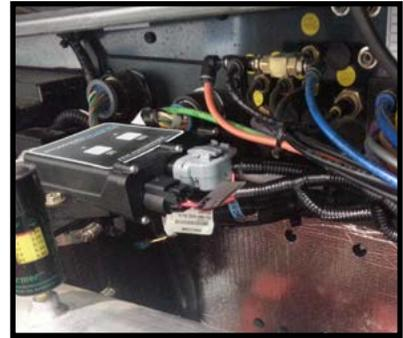
**12 |** Install the wiring harness to the PowerGuard controller and run as per the schematic provided on page 10 of this manual.
