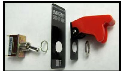
**14 |** Drill a 1/2" hole in the desired location. Route the 2 wires from the switch location to the PowerGuard controller.**15 |** Install the toggle switch through the backside of the dash, then remove the nameplate protective film and install the nameplate, switch cover, washer, and nut - as shown. Tighten nut firmly.
