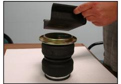
3 Using the two \%" NF x \%" capscrews, flat and lock washers, loosely fasten the assembly together. Do not tighten the capscrews fully until final adjustment is performed in step 8.
